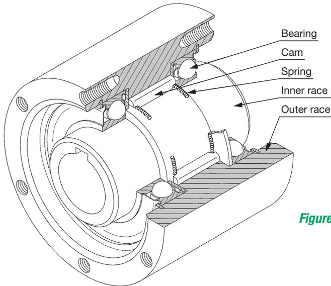
**Figure 4:** Cam Clutch major component parts
