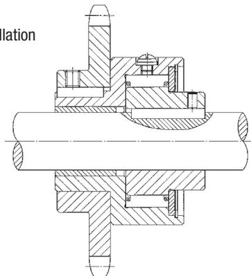
\*PBUS3 is secured to the shaft by set screw.
