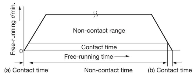
Friction in the clutch mechanism only occurs during a very short period of time denoted by “a” and “b”. “a” is the time during which the cam is engaged until the acceleration of inner race causes it to disengage. “b” is the time during which the cam engages when the inner race decelerates.
