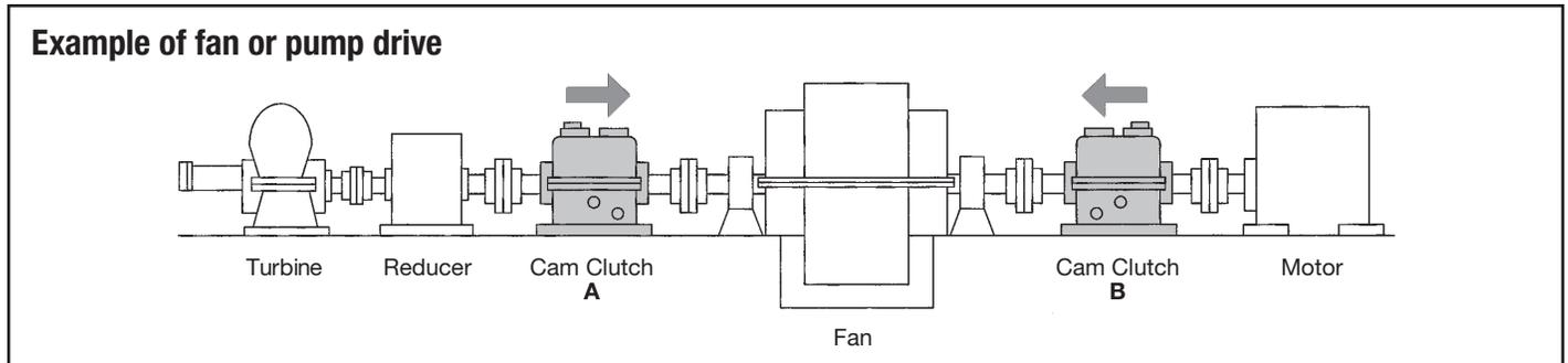
**Figure 23:** Typical High-Speed Overrunning Application
