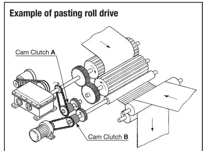
**Figure 28:** Two speed drive – Medium Overrunning and engagement
