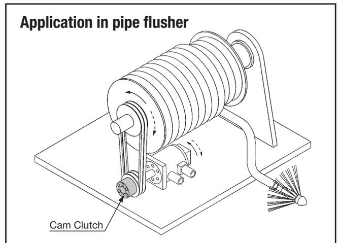
**Figure 32:** Pipe Flusher – Medium Overrunning Application
